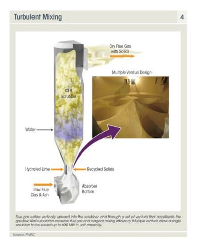
The CFBS has the ability to effectively treat more flue gas volume than an SDA. The multiple venturis present allow a single CFBS vessel to be scaled up to almost twice that of the SDA vessel option.
