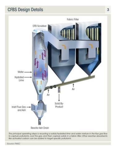
The design of the unit also provides for fast load response enabling unit cycling or load following. An added advantage is low absorber pressure drop that keeps the parasitic fan power loss to a minimum.
