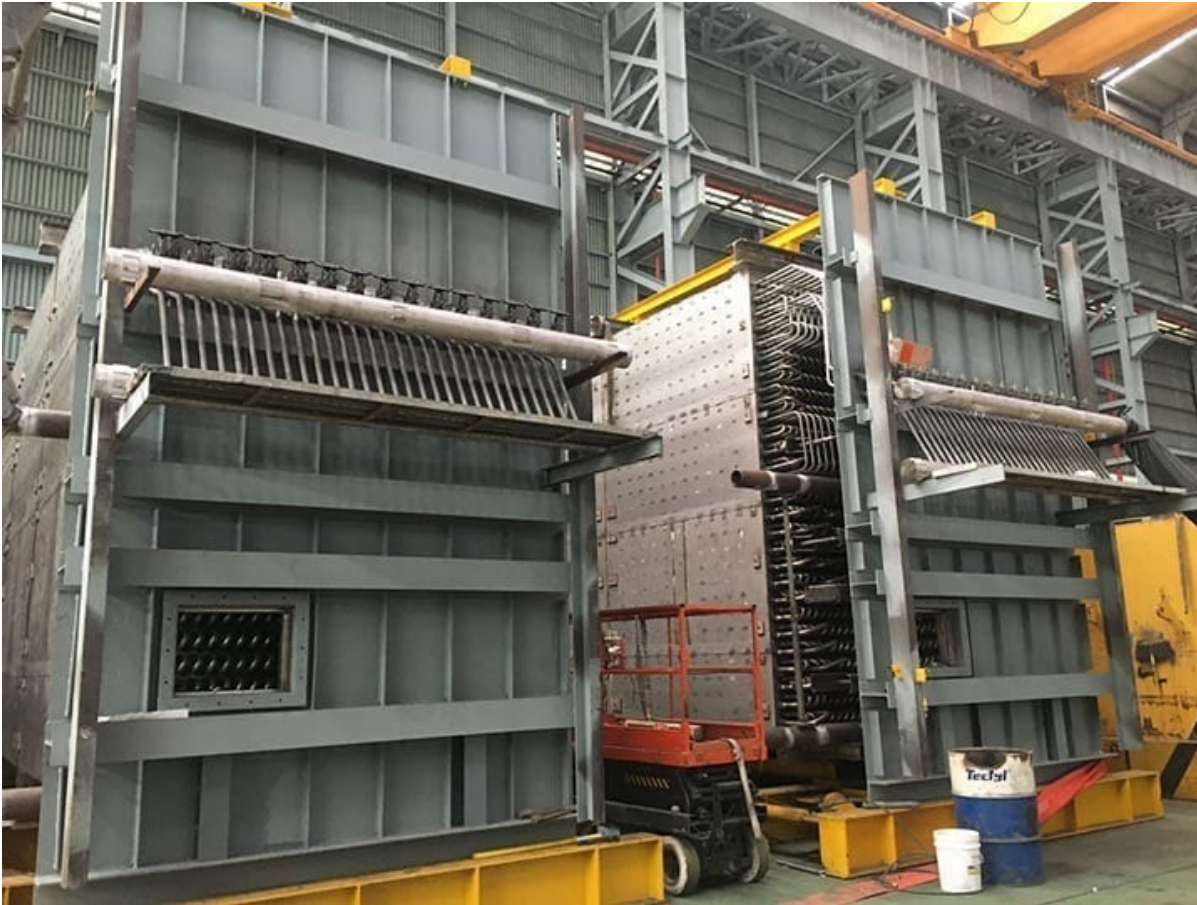
2. Fabrication of a typical vertical OTB module nears completion. The width of a single module is about 4.5 meters for shipping considerations. Note how tube sheets support the individual tubes. The modular nature of the OTB permits a very straightforward assembly sequence. Courtesy: John Cockerill Energy
