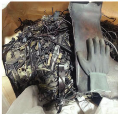
2. Debris removed from the CFB furnace when firing waste wood chips. Courtesy: Sumitomo SHI FW (SFW)
