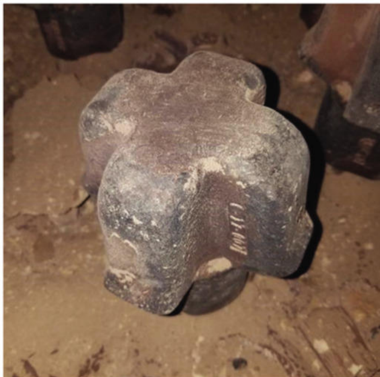
4. SFW's custom-designed changeout nozzle with variable hole sizes installed at a utility power plant. Courtesy: Sumitomo SFW
