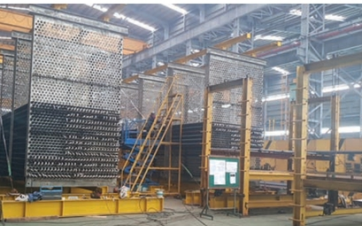
Above left: Figure 2. A typical vertical OTB module during fabrication. The width of the single wide module is about 4.5 m, an important dimension for shipping considerations. Dual-pressure OTBs are also available, with the separate serpentine tube systems arranged within a single module. Source: JCE
