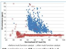
CO emissions vs GT normalised load (Source: CORMETECH)
